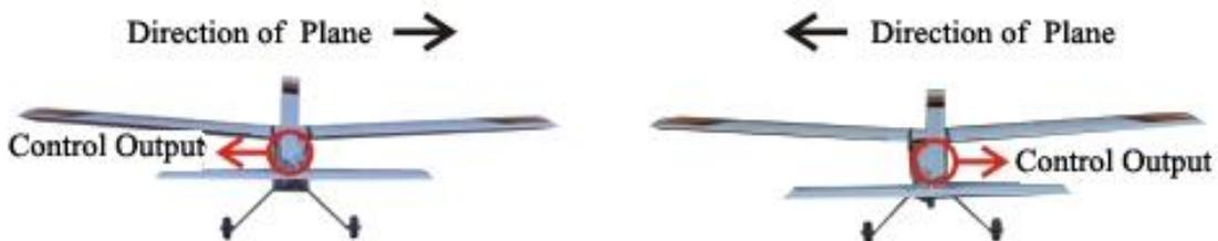
If the compensation direction is not correct, please adjust the Rudder inverse.
